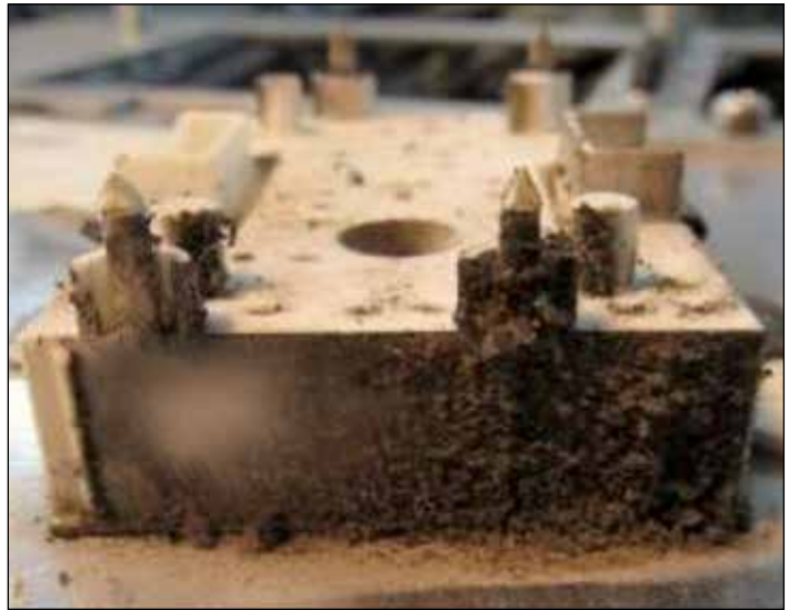
Figure 3. This close-up photo of an IGBT inside a power module shows the damage that results when dirt and dust accumulate over time, leading to overheating
