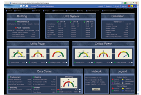
Foreseer's multiple viewing options enable companies like Verio to monitor operational status globally or to focus in on a specific site or piece of equipment.
