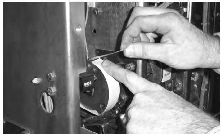
Figure 6.6. Wrapping Tape Around Cam
