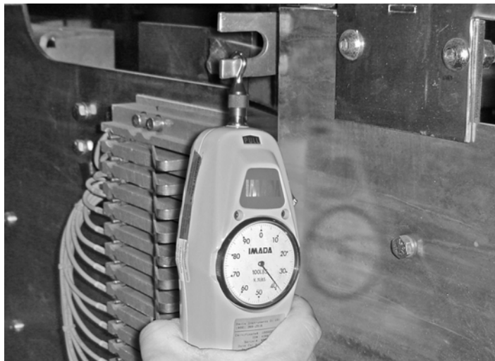
Figure 5.6. Measuring With Spring Force Gauge
