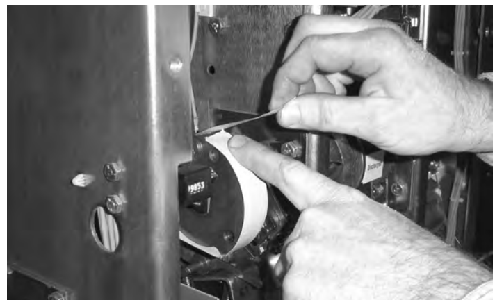
Figure 6.6. Wrapping Tape Around Cam
