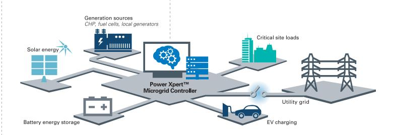
The microgrid controller maintains overall system stability regulating power flow and monitoring protection schemes in real-time, while dynamically managing generating assets and loads to meet user defined goals.
