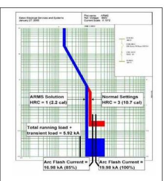
Figure 3 – Time-Current Curves showing Trip Time with Energy-Reducing Maintenance Switching [10].
