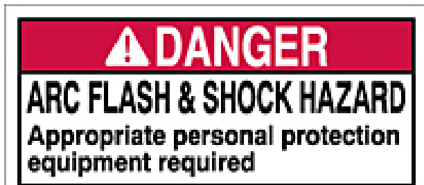
Fig. 1. Example of an Arc-Flash Hazard Warning label per NEC [2], Section 110.16
