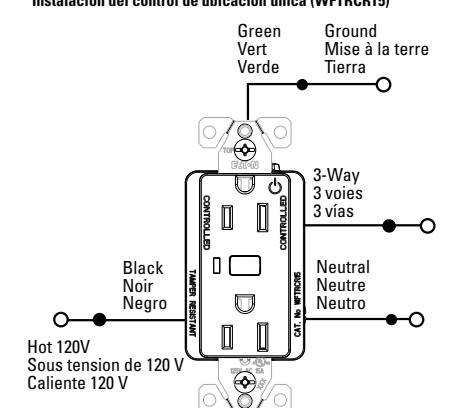
**Two Location Control Using a 3-Way Switch**
