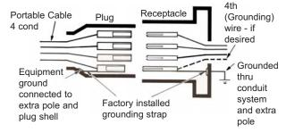
Style 2 units with a metallic housing have an extra (grounding) contact which forms a parallel circuit with the circuit formed by the plug sleeve and receptacle detent spring.
