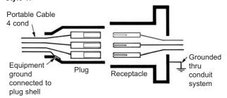
Style 1 units ground the portable device and the plug via the grounding conductor and the plug shell to the receptacle housing. The receptacle is grounded by virtue of its being and integral part of the conduit system.
