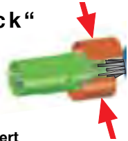
Fig. 14.5 Fit divided insulating sleeve
