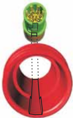
Fig. 8.4 Fit connector insert
