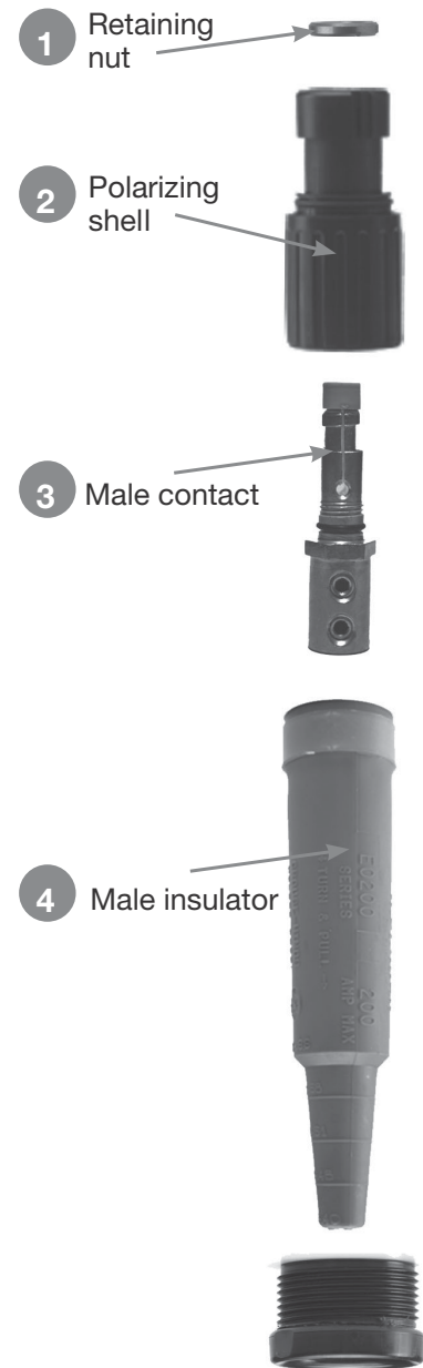
Male plug assembled length is 8-3/4"
