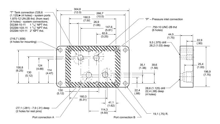
♦ Manifolds or other mounting interface can be drilled to 33,3 (1.312) dia. Fitting size and fitting spacing limit the subplate port size to 28,6 (1.125) dia.
