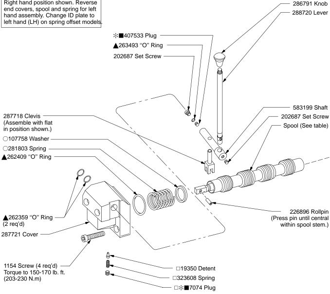
□Use with No-Spring Detented models. Omit for Offset and Spring Centered.
