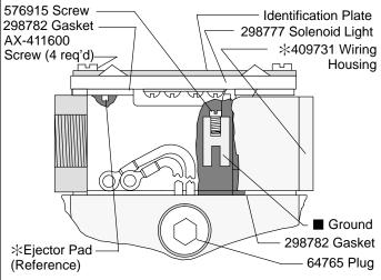
Assemble with circuit breaker and light over solenoid.
