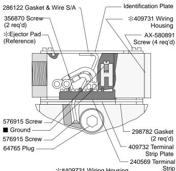
\*#409731 Wiring Housing Assemble housing with ejector pads ip and with electrical conduit connection over solenoid "B". (Solenoids "A" and "B" are identified on units by diagram plate on side of pilot valve. For type "4" and "8" spools conduit connection location on
