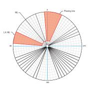
The circular close permits the network protector to close at lower loads while assuring the watt flow is into the network.
