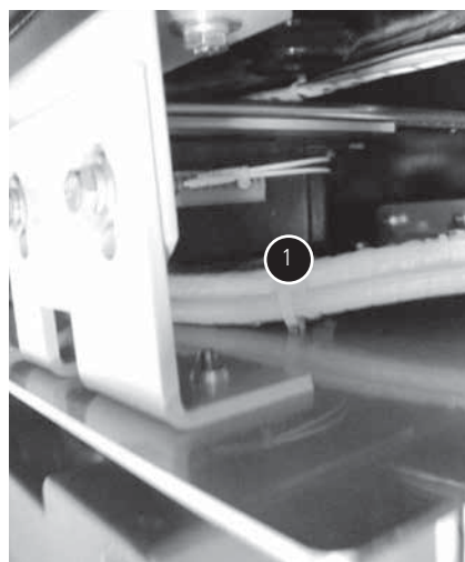
Figure 6. Wire Bundle Side Attachment
