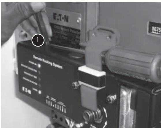
① Remove small cap and depress button start programming. Learn Mode LED will illuminate.
