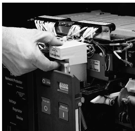
Fig.14 Removing Spring Release
