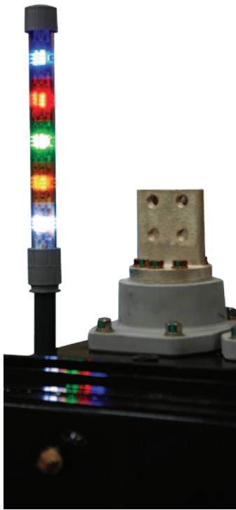
Figure 3. Network protector shown with optional IP68 rated submersible stacklight. The LED colors are: Flashing Blue = NPArms mode, Red = Close, Green = Open, Yellow = Racked out to test position, White = Racked in or connected to energized bus.
