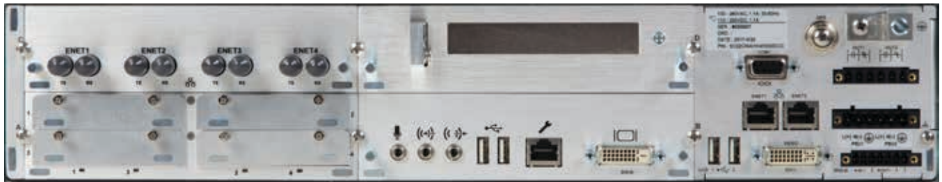
Figure 2. SMP SC-2200 platform - rear panel (with Ethernet, Drive Bays, PCIe adaptor, and PC modules)
