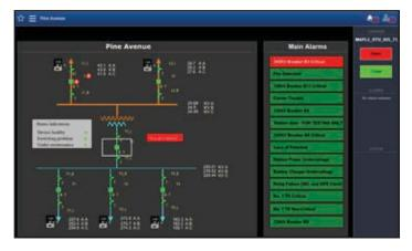
The control command inhibition button, which is used for local/ remote status protection, is an example of an object often used in a substation single-line diagram page. This control interlock mechanism toggles the control operation mode, local or remote, of the substation gateway. This is very easy to configure with the use of the substation gateway internal system data point.
