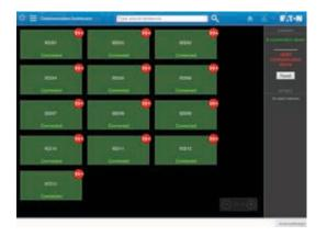
with a quick overview of the communication statuses of all IEDs configured in the substation gateway in a single page, as well as control center communication links. A summary and details pane, as seen in the right side of the second image, displays summary connection statistics and detailed statistics related to the selected communication link; reset operations are allowed on the latter.
