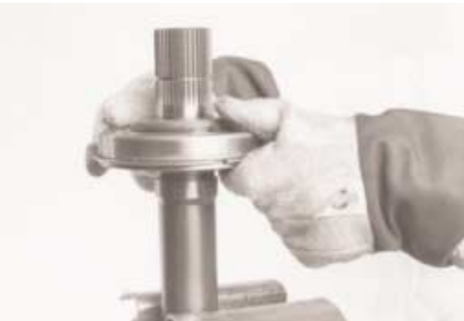
2. Place the input shaft in a vice. Heat the bearing sub-assembly to 120°C and fit it onto the shaft.
