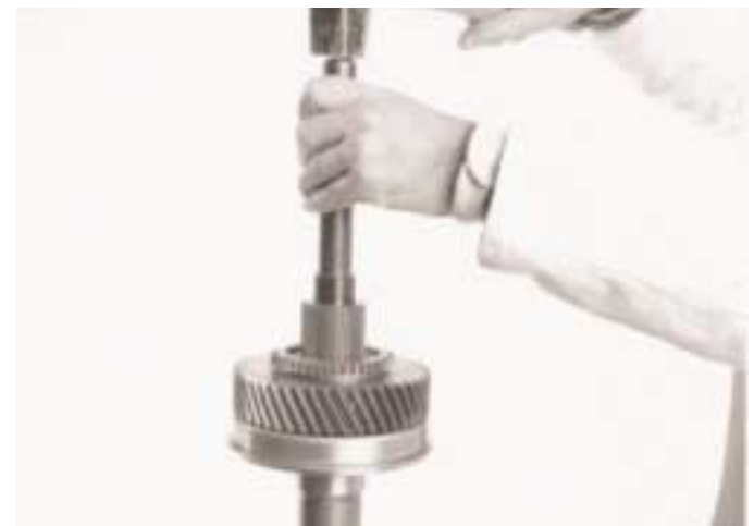
6. A new bush can then be fitted using tools E 109 and E 109-15.
