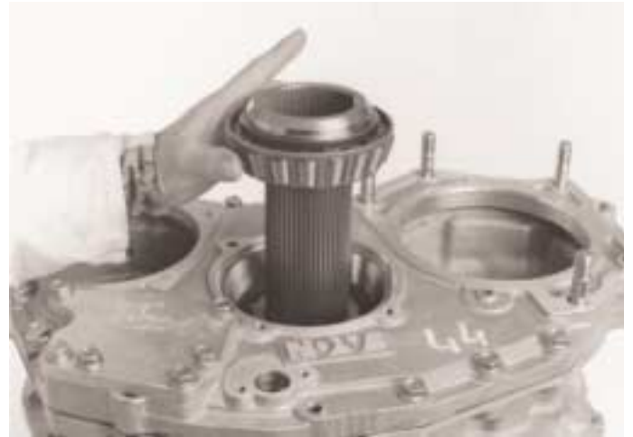
13. Refit the bearing/spacer assembly.
