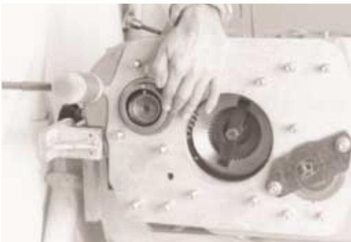
14. Remove the tool E 207 from the upper countershaft. Remove the bearing outer.
