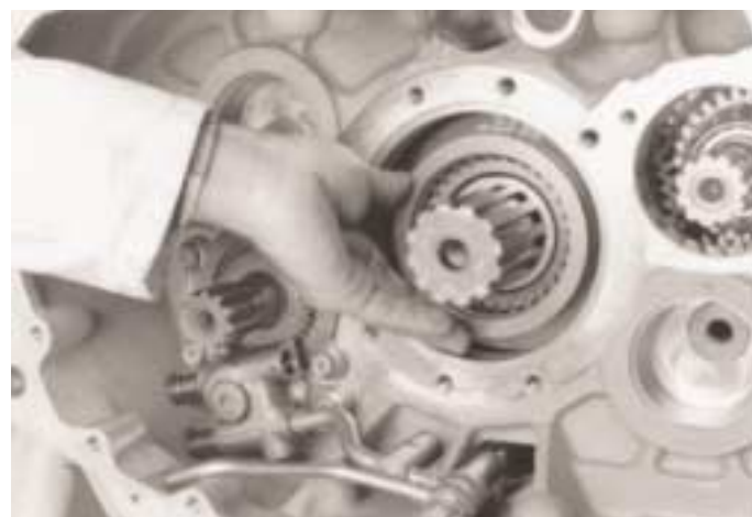
20. Refit the reverse gear sliding clutch, boss forward, onto reverse gear splines.
