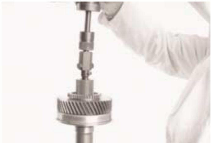
5. If damaged, the input shaft bush can be removed using tools MS 284 and MS 284-1.
