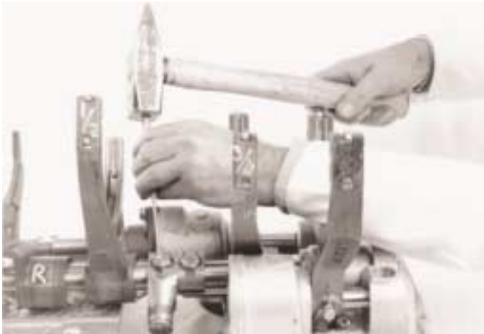
6. Refit the shift finger, tab washers, screw and nut.
