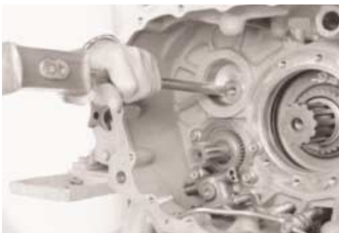
18. Drive the reverse idler shaft forwards until it is flush with the maincase face.
