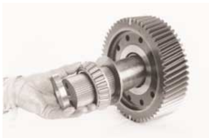
20. Remove the spacer. If necessary use a press or puller to remove bearing and thrust washer.
