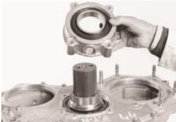
11. Remove speedometer housing assembly.
