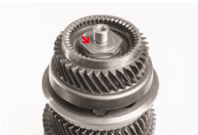
Mainshaft spindle - M22 285 to 315 Nm
