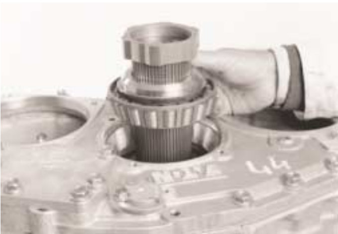
12. Remove the speedometer rotor and bearing/spacer assembly.
