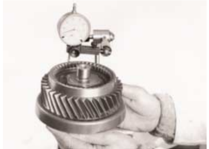
15. Place mainshaft in a soft jawed vice. Using a dial test indicator measure the 4th speed gear end float.
