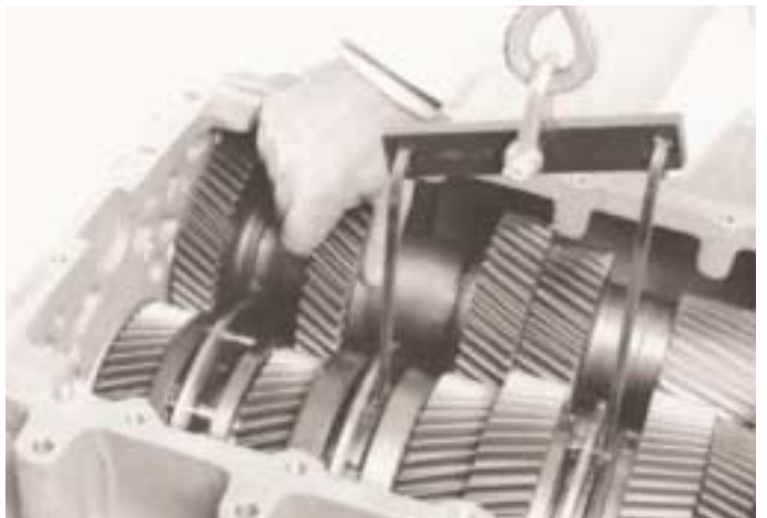
24. Remove the tool E 201 from the countershaft. Rotate the upper countershaft until the timed teeth of the input shaft gear and countershaft gear are in mesh.
