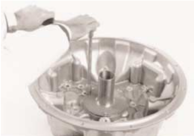
1. Place the clutch housing on a bench and refit the front cover.
