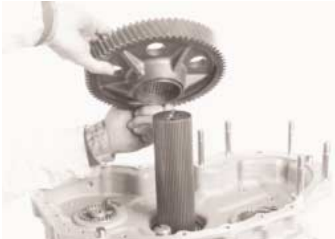
10. Refit the drive gear, boss down.
