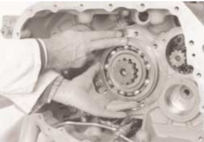
22. Refit mainshaft rear bearing and spacer assembly.
