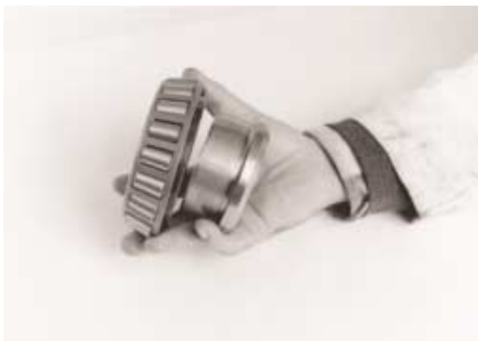
13. The bearing can be pressed off the spacer if necessary. Heat the bearing to 120°C before refitting.
