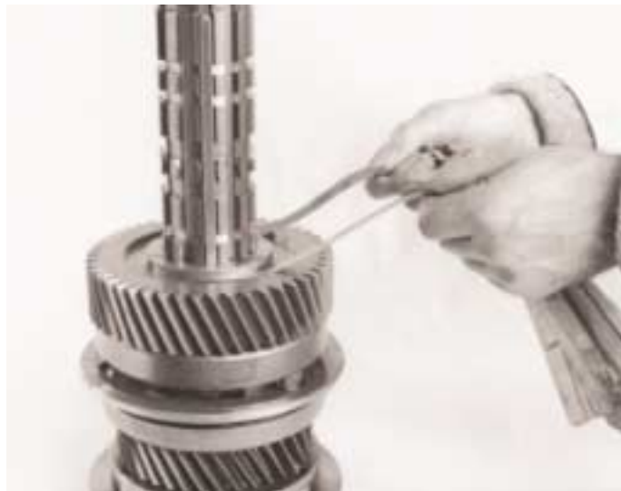
11. Refit the mainshaft key. Using feeler gauges measure 3rd speed gear end float.
