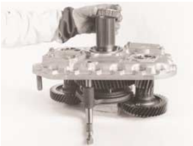
13. Heat the bearing to 120°C and refit to the output shaft.
