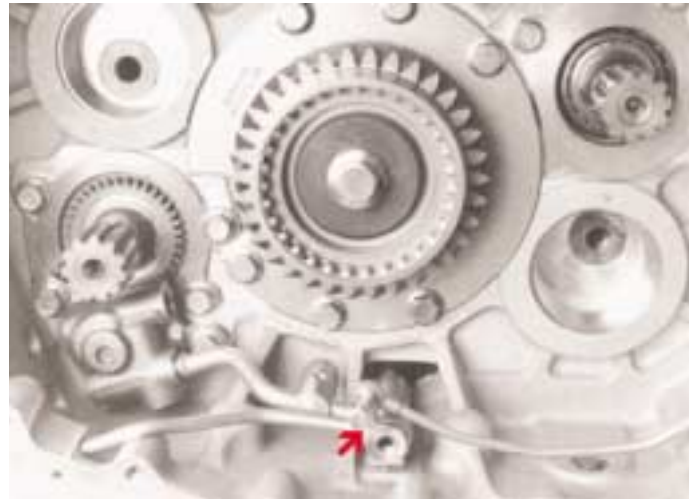
3. Remove oil feed screw and pipe.
