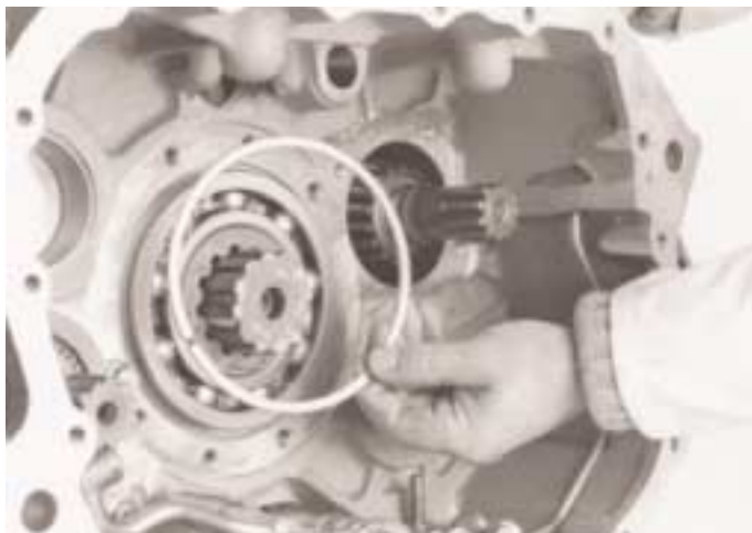
20. Pull the mainshaft rearwards to expose the bearing snap ring. Remove the snap ring.
