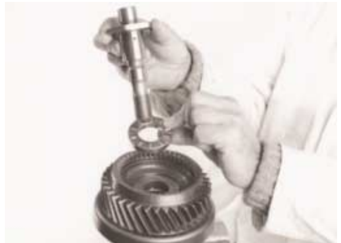
16. Remove mainshaft spindle and bearing.
