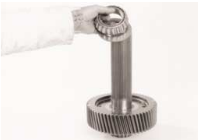
26. Using a press or puller remove bearing and thrust washer.
