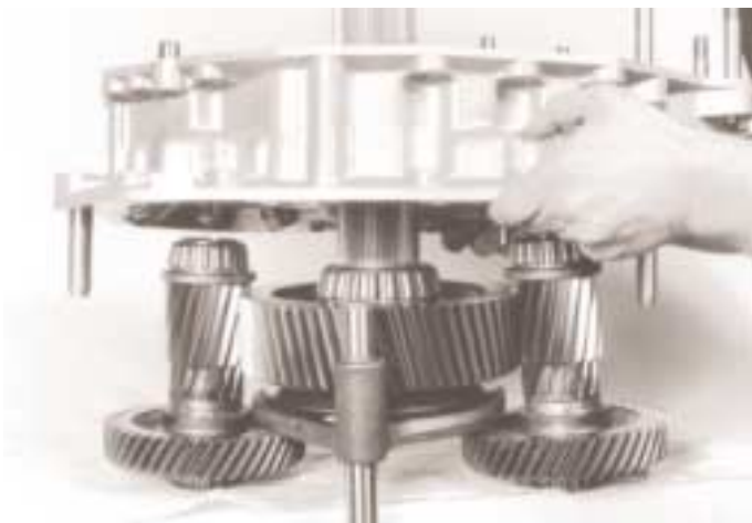
17. Remove the auxiliary housing.
