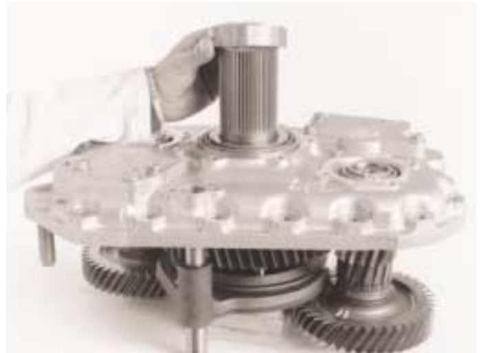
14. Refit the speedometer rotor.
