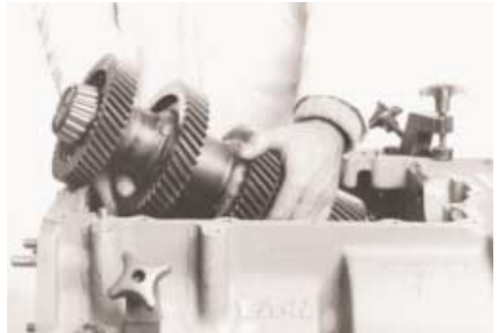
28. Remove the upper countershaft assembly. The countershaft assemblies are assembled and welded during production. Therefore apart from the bearings there are no serviceable parts.
