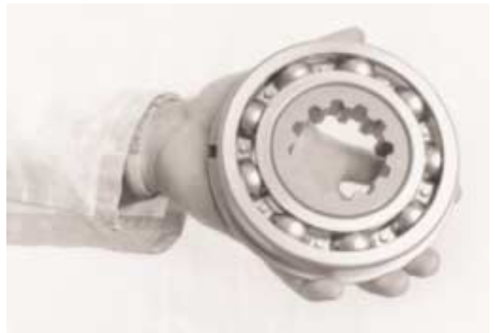
22. If necessary the bearing can be pressed off the spacer. If replacement is necessary, heat the bearing to 120°C before refitting.
