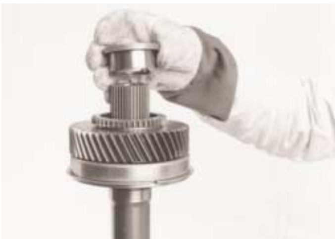
3. Place the gear on the input shaft, clutching teeth up. Heat the sleeve to 120°C. Fit the sleeve to the shaft.
