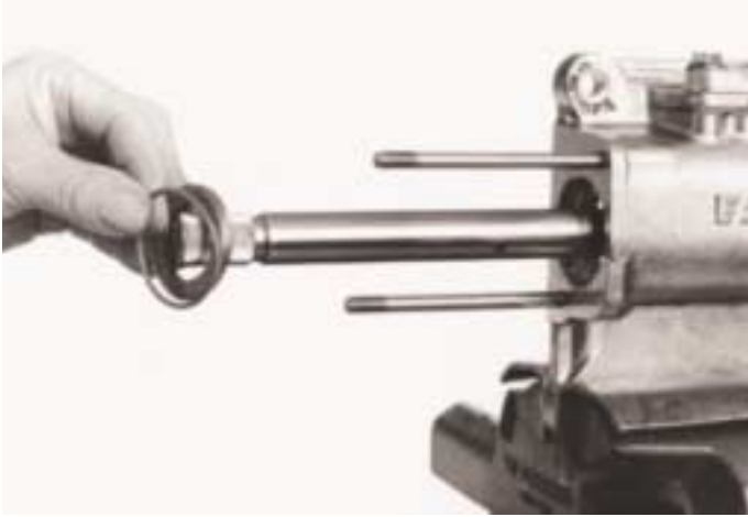
6. Remove O-ring and washer.
