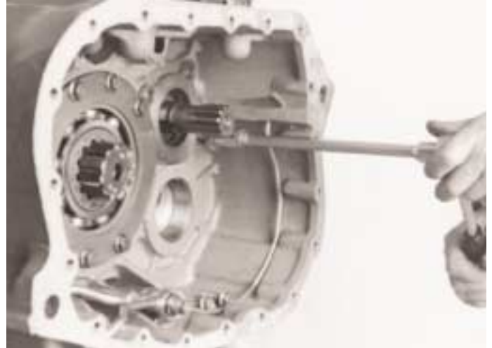
11. Remove the screws from the upper countershaft bearing support.
