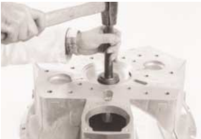
2. Turn the clutch housing over and use tools E 109 and E 109-19 to fit a new oil seal if necessary. The flat face of the seal must face the front cover. Drive the seal in until flush with the rear face.
