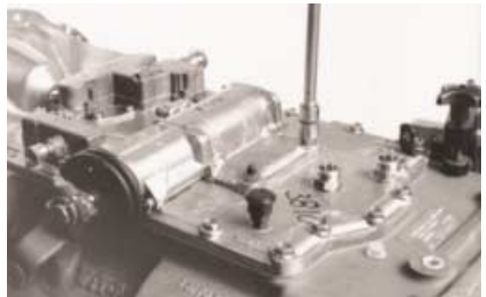
10. Refit remote control to shift bar housing. Refit reaction rod and bracket.
