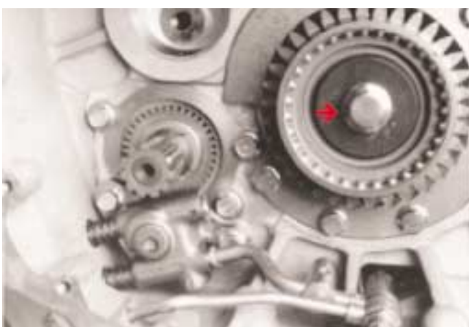
Mainshaft gear retainer - M16 230 to 250 Nm
