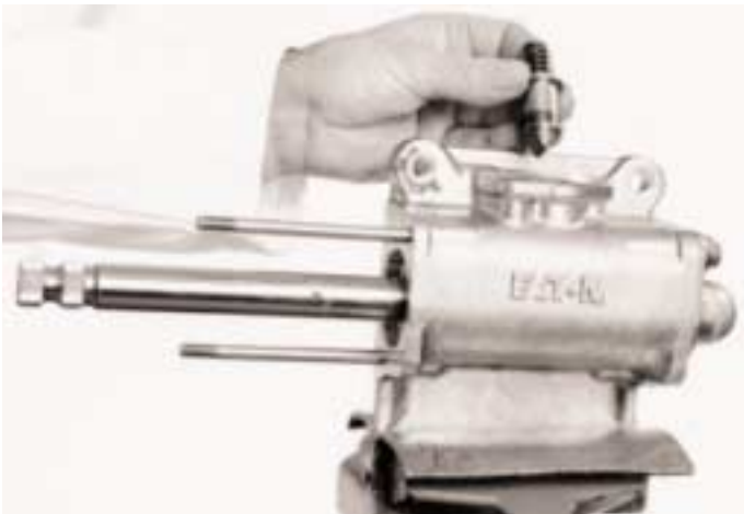
7. Remove detent plate, gasket, spring and plunger.
