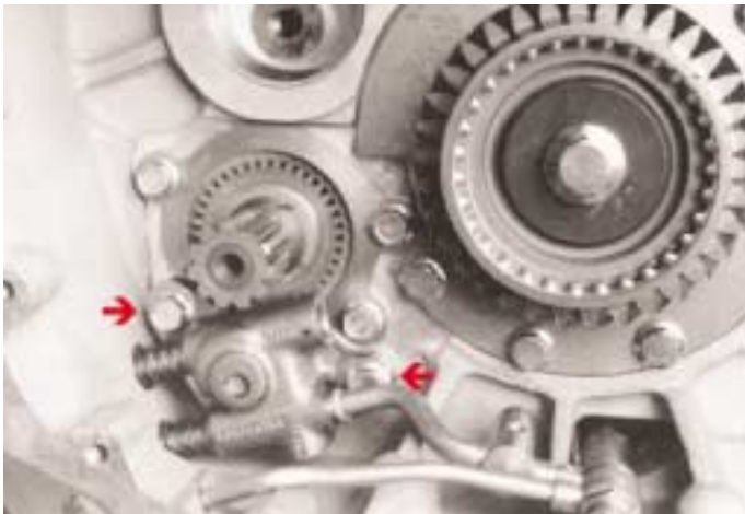
Oil pump housing - M10 70 to 80 Nm
