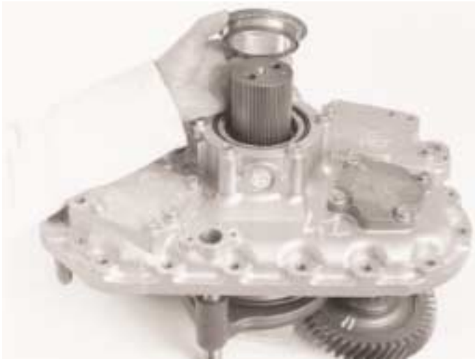
16. Refit the speedometer housing inner oil seal/spacer assembly.
