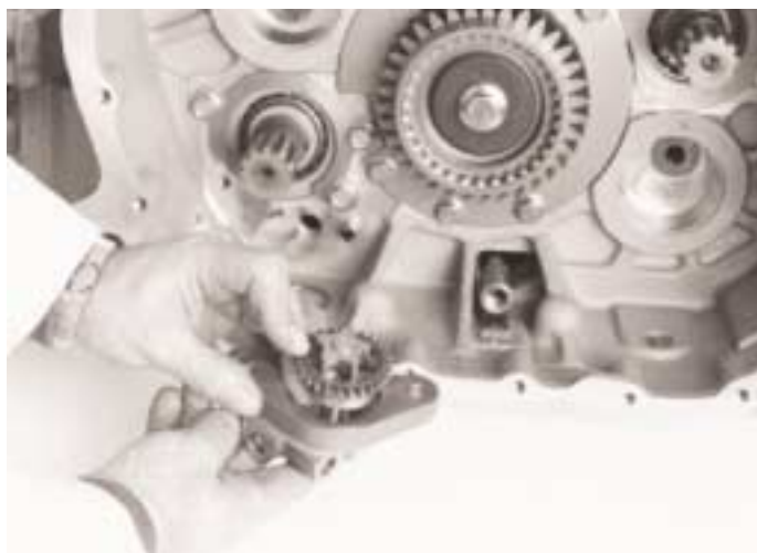
7. The oil pump consists of a gear and a rotor.
