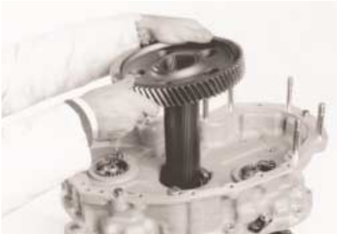
16. Remove the drive gear for the Voith retarder.
