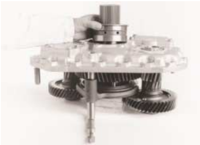
12. Lower the auxiliary housing onto the components ensuring that the auxiliary countershafts and the range change shift bar are seated in their respective bores. Refit the bearing outer.
