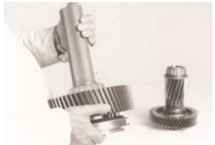
19. Identify the left and right hand auxiliary countershafts. The two auxiliary countershafts and the output shaft assembly can now be removed.
