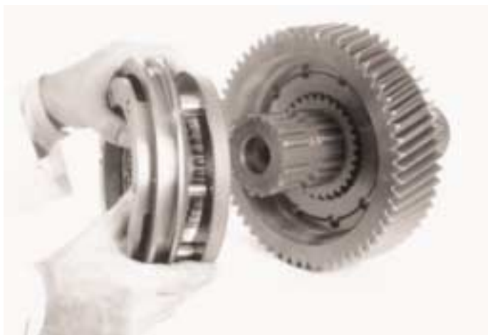
19. Remove the range change synchroniser assembly.
