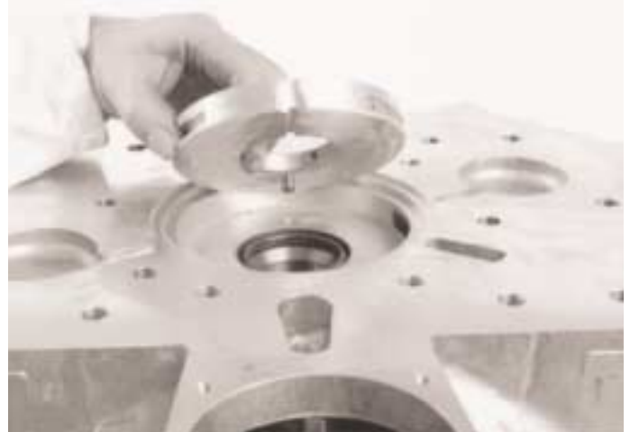
3. Refit the lubrication plate ensuring that the dowel is correctly located in the hole in the clutch housing.
