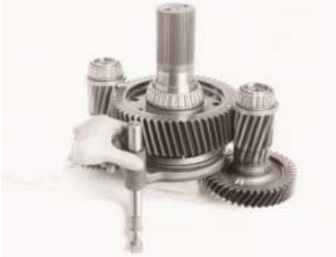
11. Refit the range change shift bar and fork assembly.
