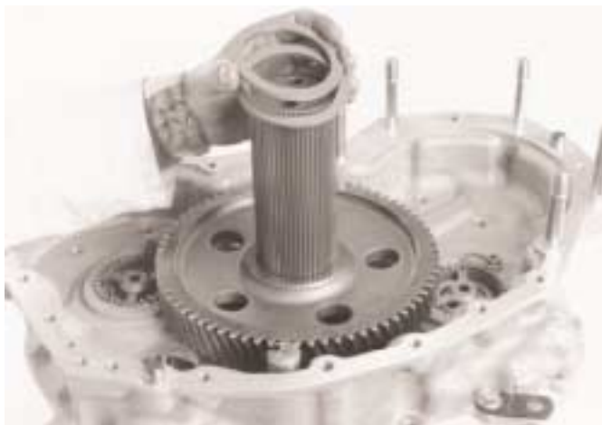
11. Fit the two graded spacers. These are used to set the bearing end float.
