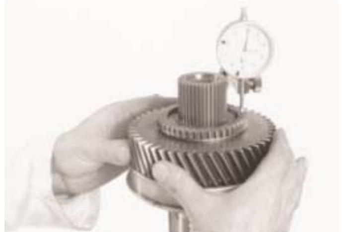
4. Allow the components to cool. Refit the snap ring and then check that the gear end float is within the specified limits.
