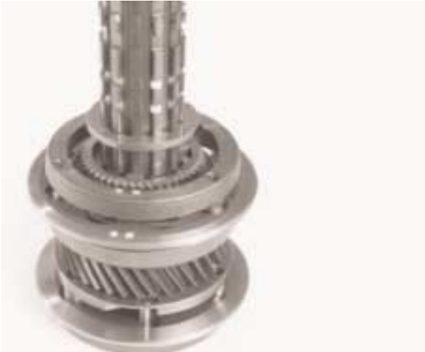
13. Identify 3rd/4th synchroniser assembly and orientation.
