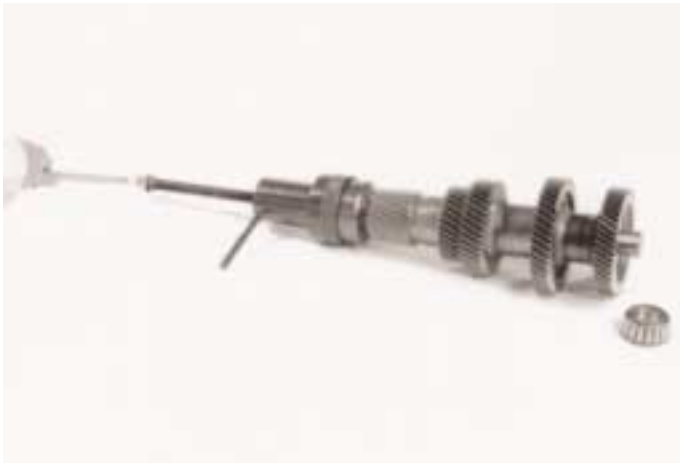
29. The bearings can be removed from the countershaft using tools LC 105A and E 105-4. If the bearings are changed the corresponding outers must also be changed and vice versa.
