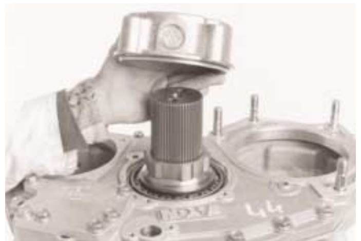
14. Refit speedometer rotor. If the O-ring on the speedometer housing is damaged, replace it and refit speedometer housing.
