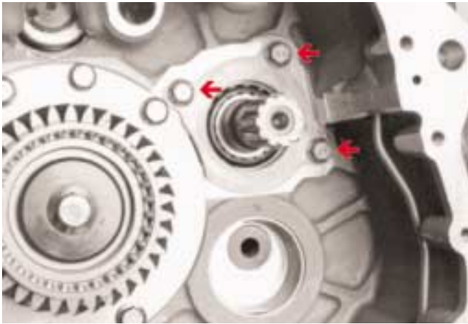
Countershaft bearing retainer - M10 70 to 80 Nm
