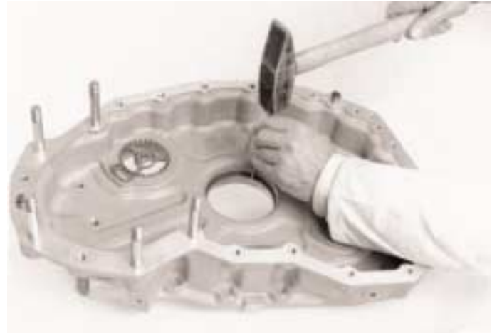
28. If either of the output shaft bearings need replacing, the corresponding outers must also be replaced. The outers can be tapped out from the auxiliary housing or rear plate.
