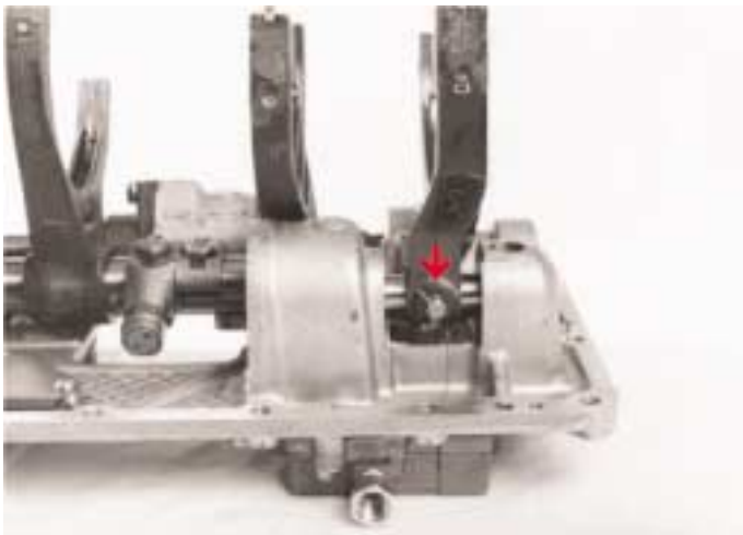
Splitter fork lockscrew - M10 10.5 to 12 Nm with Loctite 265
