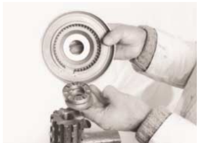
17. Remove 4th speed gear, bearing and thrust washer.
