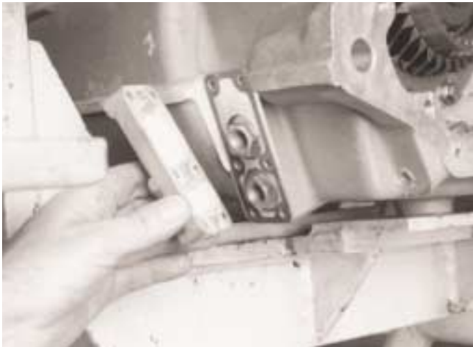
1. Remove oil transfer plate and gasket.
