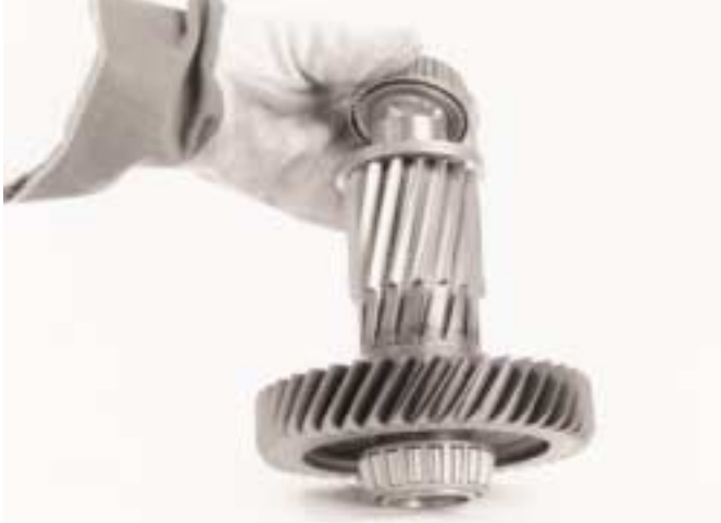
24. When replacing the bearings heat them to 120°C before fitting.
