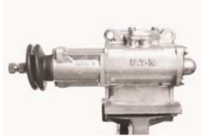
8. Refit rubber boot with drain hole pointing down.
