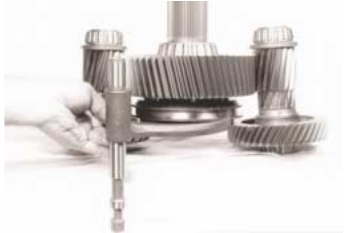
18. Remove the range change shift bar and fork assembly.
