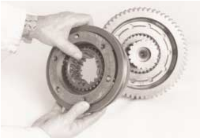
25. Remove the range change synchroniser assembly.
