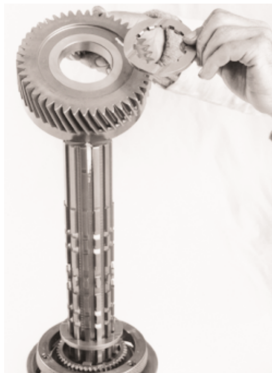
12. Remove mainshaft key, thrust washer and 3rd speed gear.
