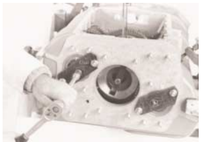
12. Mark the position of the taper bearing assemblies. Use the centre screw on the tool E 207 to push the upper countershaft rearwards approximately 5mm. This gives access to the rear bearing support.
