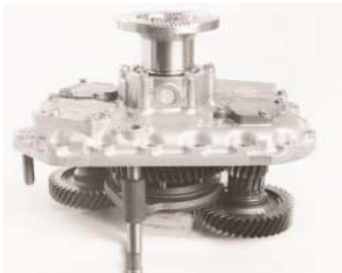
17. Refit the coupling flange, retainer plate and screws.
