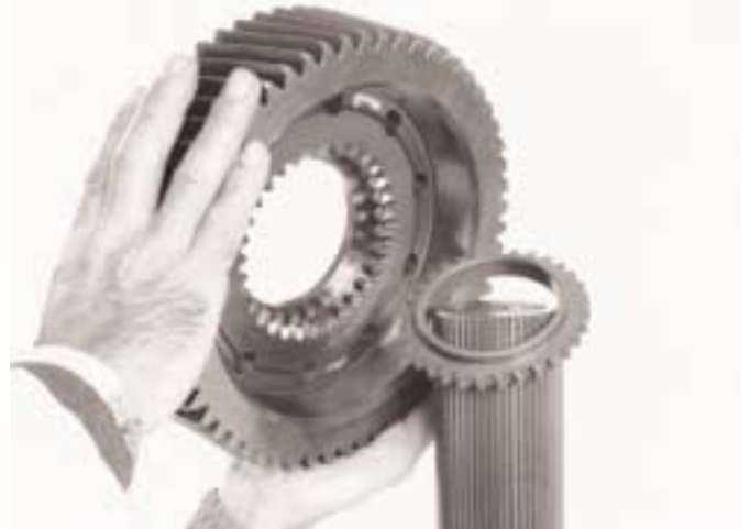
27. Remove the low gear and the splined washer from the output shaft.
