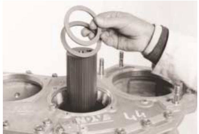
14. Remove the graded spacers.
