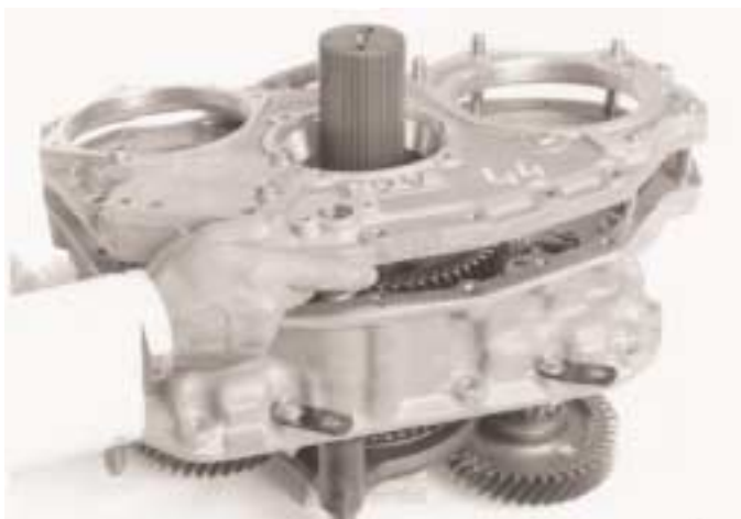
12. Fit the gasket, apply sealant and fit the rear plate.
