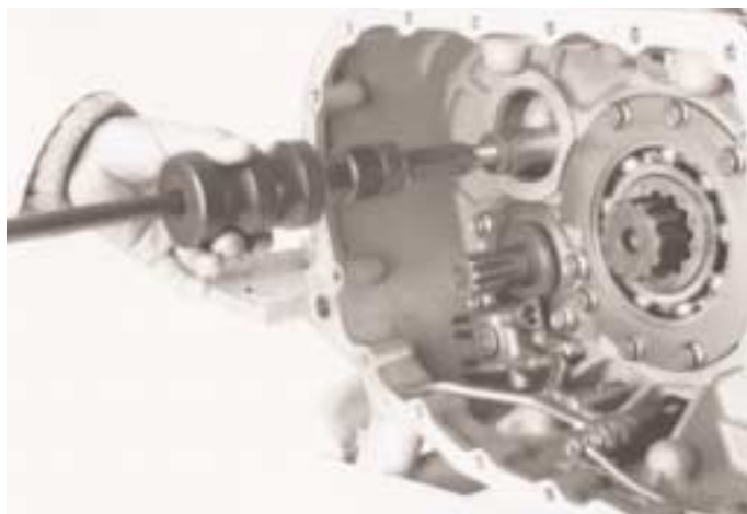
17. Remove the reverse idler shaft using tools MS 284 and E 200. The thrust washers and spacers on the idler shaft will drop into the main case.
