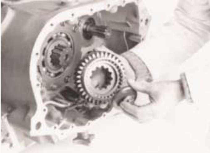
9. Remove the screw, retaining plate and auxiliary drive gear.
