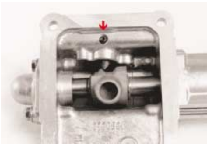
Remote control screw - M5 3.5 to 4 Nm
