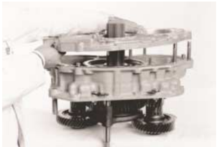
15. Remove screws and lift the rear plate off the locating dowels. Remove gasket. Remove locking plate.
