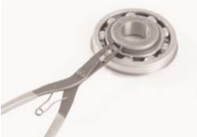
1. Place the sleeve on the bench. Fit the bearing and the snap ring.
