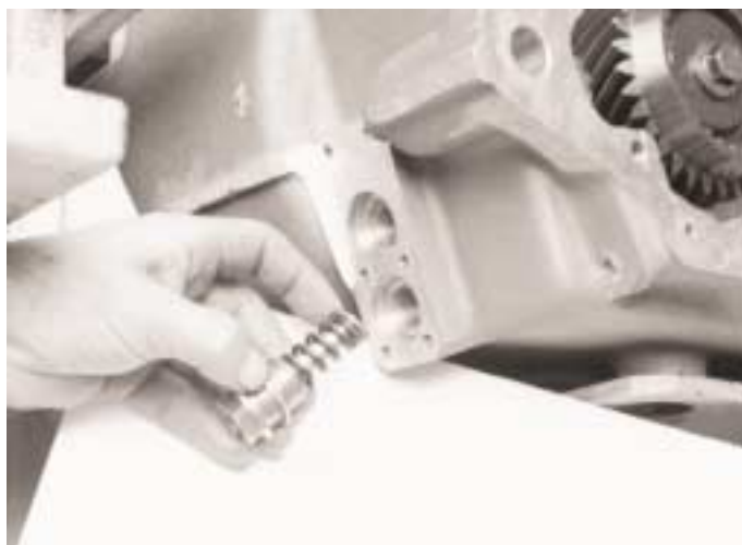
2. Remove oil feed pipe, washer, spring and washer from both positions.
