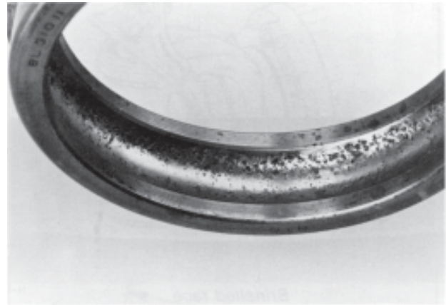
Burnt and Spalled Bearing
