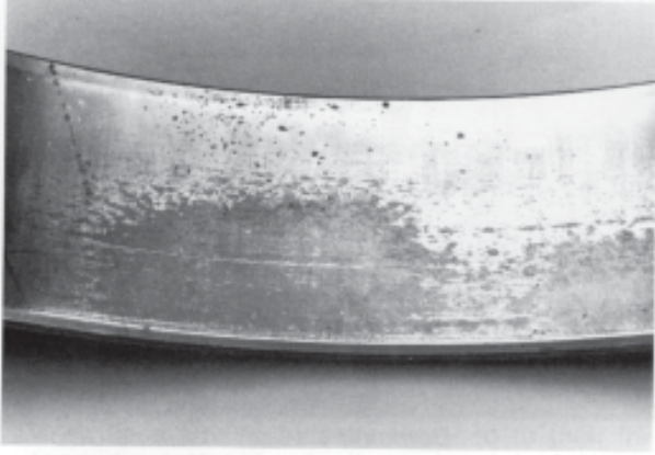
Bearing Race "Flaking"
