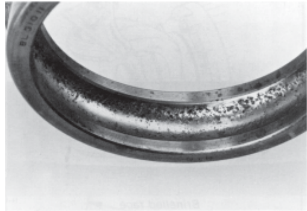
Burnt and Spalled Bearing
