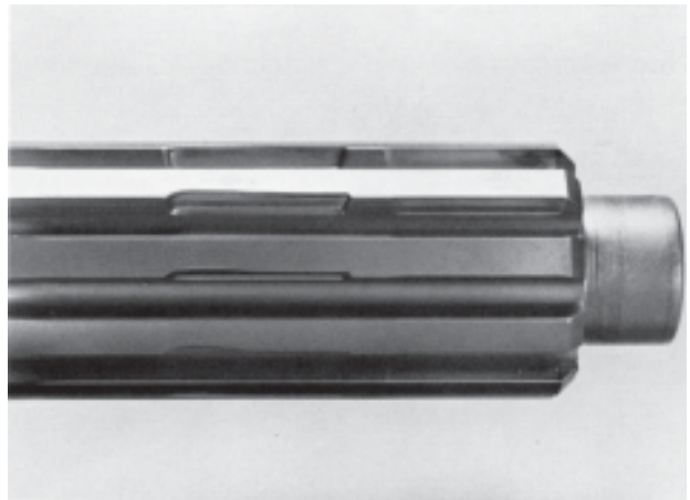
Input Spline Wear
