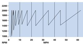
Based on engine operating at 2000 RPM with top geared road speed of 62 MPH.
