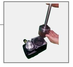
**13.-** Once the DIN 912 M5x16 three screws are loosen, extract the Piston Housing by hand.
