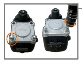
**31.-**Mount the washers and the M12 Nuts. Tighten with pneumatic screwdriver tool.
