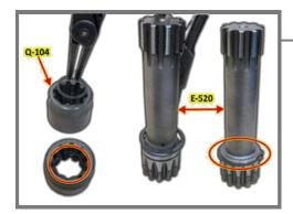
**40.-**Mount the corresponding Circlip on Q-104 and on Shaft E-520.
