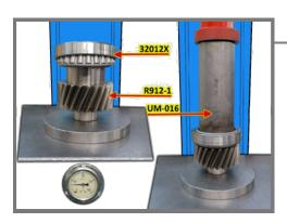
**3.-**Put the Taper Roller Bearing 32012X in R912-1 upper gear. Press with tool UM-016 at 30 ±5bar.
