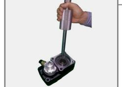
**10.-**Once extracted the circlip, we will proceed to thread a special inertia extracting tool on the M12 shaft thread.
