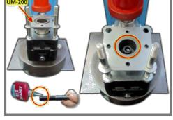
**38.**-Assemble the washer and bolt into transmission Flange and tighten it at 80±5 Nm.
