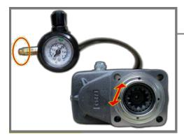
**29.-**Remove inlet air pressure and wait for about 20"-30", verify that pressure gauge needle doesn't move. Ensure that the displacement is the correct one.
