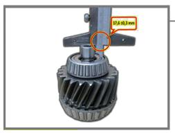
**19.-**Verify that measurement shown on image is the correct one (17,6 ±0,3 mm).
