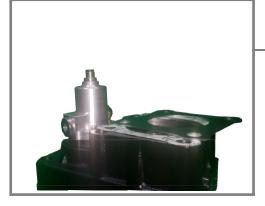
**5.-**Once extracted the flange, we will proceed to loose the seal stop plate.
