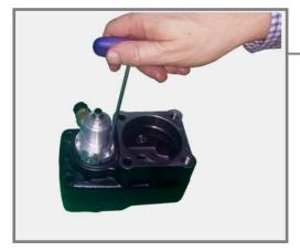
**14.-** Remove the T285 Cover of the Central Piston.
