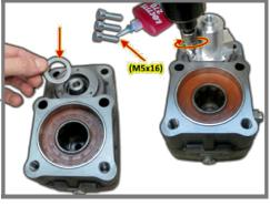
**27.-**Thread two metallic Plugs in both lateral holes of piston Cover. Connect the air flow regulator and inject air (5.7 bar approx.).
