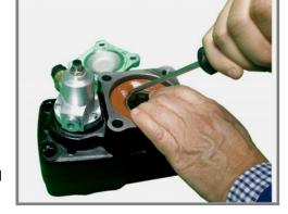
7.-Poke a screwdriver into rubber part of the Seal and continue with disassembling by pulling out the seal.
