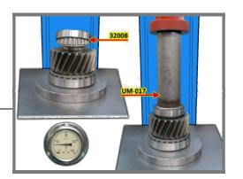
**4.-**Turn around the upper Gear and collocate the Taper Roller Bearing 33008. Press with tool UM-017 at 30 ±5bar.
