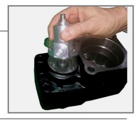
**15.-** Remove the X221 Screw for Central Piston. Use an impact gun to do it easier.
