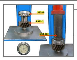
**1.-**Put the Taper Roller Bearing 32209 in R911-1 bottom gear. Press with tool UM-002 at 30 ±5bar.
