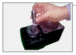
**16.-**Extract by hand the Washer, Spring and Guide for screw.
