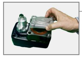
**3.-** Remove the Blank Cover and the Gasket.
