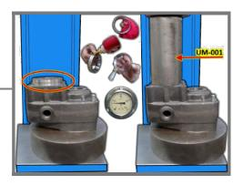
**9.**-Clean up glue residue. Then mount the circlip Ø85.
