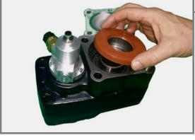
9.-We need to extract the circlip DIN472 Ø85 that is fixing the bearing.
