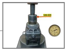
23.-Next step: Assembly of the pneumatic Piston.
