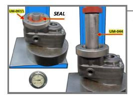
**13.-**Position the tool UM-097/1 and collocate the Seal (45x85x10) with lips looking down. Centre in its place and press with tool UM-044 at 8 ±2bar.
