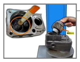
**7.-**Apply grease on 32007 bearing race interior. Introduce the bottom Gear R911-1 on PTO Housing as it's shown on image.
