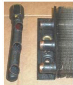
Copper Cooler Failure
