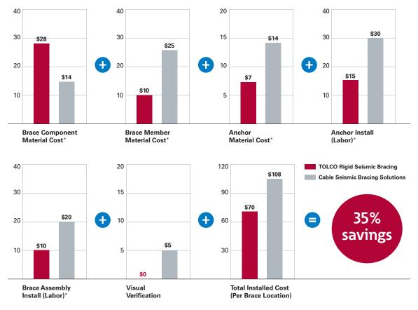
\* Material costs shown are based on average prices of TOLCO rigid seismic brace attachments, Eaton B22 Strut as the brace member, and standard generic cable attachments. This also includes u-clips, thimble and pre-stretched aircraft cable as the brace member. Labor rates shown are estimated using average 2013 union labor rates from regions of the U.S. where seismic bracing is typically required, as well as average observed installation times.
