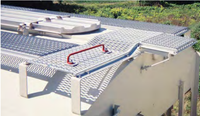
Grip Strut railcar walkways
