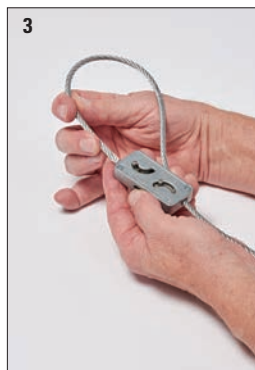
3 Pass wire rope back through KwikWire Clamp
