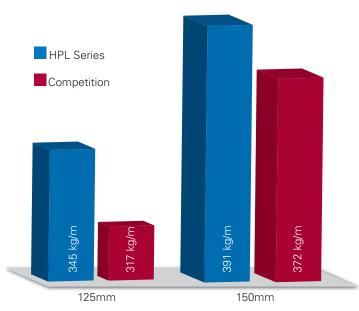
The High Performance Ladder (HPL) Series is a patent-pending high performance cable ladder that reduces weight while increasing load capacity. Designed to literally save tons in overall weight on offshore and modular construction applications, the HPL cable ladder offers a unique combination of low weight and high strength. The high strength to weight ratio allows for increased load capacities and helps keep weight budgets in balance.
