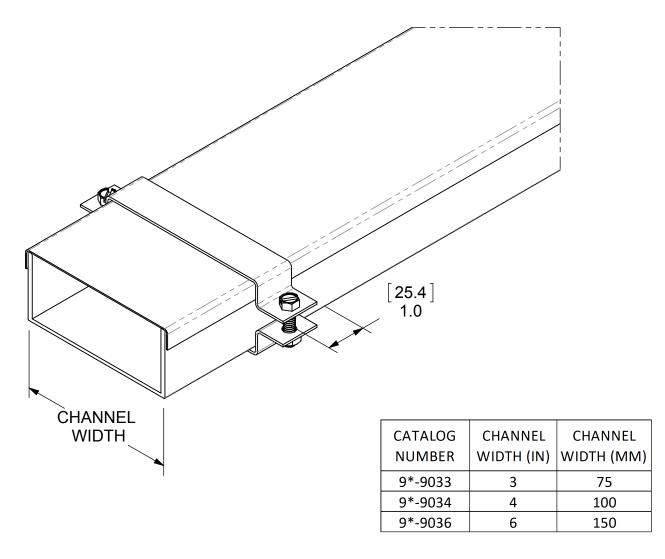
HARDWARE: 1/4-20 x 3/4" HHMS - 2 PC. 1/4-20 HEX NUT - 2 PC. \* - P = PRE-GALVANIZED STEEL A = ALUMINUM G = HOT-DIP GALVANIZED SS4 = 304 STAINLESS STEEL SS6 = 316 STAINLESS STEEL
