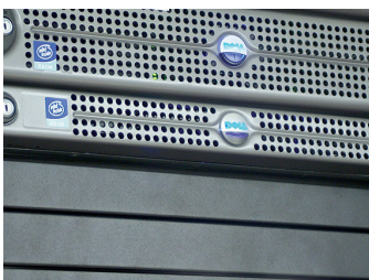
Blanking panels provide a quick, easy and cost effective solution to optimize air circulation within an enclosure.
