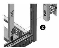
3 Install and slide down to capture into slots.
