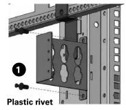
Align plastic mounting buttons with keyhole slots on ePDU brackets
