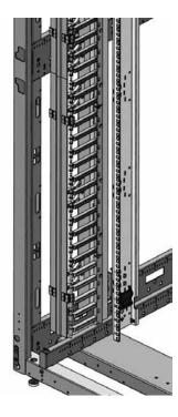
1 Install ePDU 90 mounting brackets to side of rack rail.
