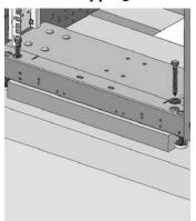
Using a %6 socket, remove the four shipping bolts and washers that anchor the enclosure to the pallet. Also remove spacer board from under frame before moving enclosure from pallet
