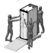
Ramps (RSRMPSTD ordered separately) are available to assist in removing the enclosure from the pallet.
