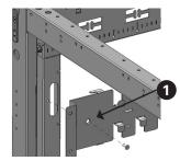
1 Install mounting bracket in top location on frame. Screw with #6 screw.
