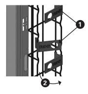
Gates come in kit of left hand and right hand and simply snap on Flextray wire.
