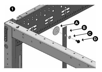
Assemble as shown; note location of isolation washer.
