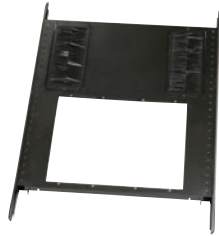
Top panel includes two brush strips for cable entry. Brush cable openings can accommodate 1,000 (42"D) to 1600 (48"D) CAT6 cables. Model JTPTC3045 shown here.
