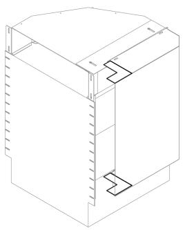
8. Fabricate the two plastic sheets as needed to form the best seal between the top and bottom of the side intake and the rail. Affix the fabricated seals.
