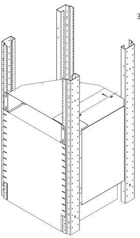
3. From above or below, position the side intake next to the switch between the right side rails. Make sure the switch intake is closely aligned with the side intake of the airflow director.
