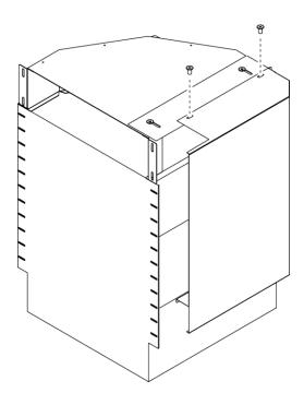
5. Insert two 10-24 screws through the slots on top of the side intake into the connecting plate and tighten.
