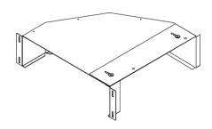
**Note:** The two screw holes in the connecting plate must be on the right side, with the holes closer to the rear, as shown.
