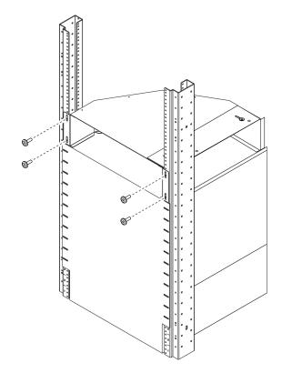
2. Using the included fasteners, insert four screws and/or nuts as needed to attach the top intake to the rails.
