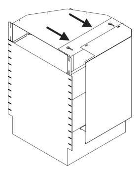
4. Slide the adjustable connecting plate under the top of the side intake. Align the slots in the top of the side intake with the screw holes in the connecting plate
