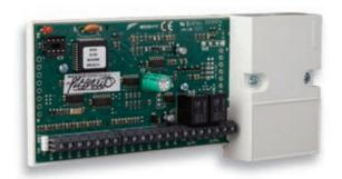
The 8400 is a wired, auto-dialling digital communicator, capable of being programmed to support monitored installations that require a police response.
