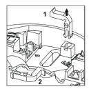
Mount the sensor onto the base and rotate fully clockwise until it finally clicks
