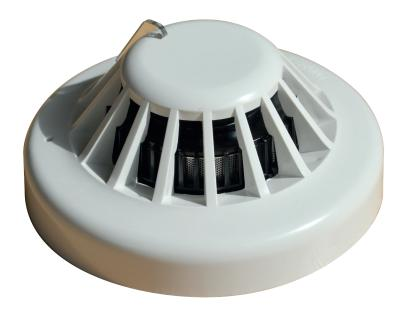
The BiWire Ultra range offers a multi-mode, 5 in 1 detector, approved to both EN54 parts 5 & 7, which covers many building needs. It's quick and simple to install with a stylish low profile design. The detector is mounted on our standard conventional base (FXN520). Each detector is fitted with a 360° viewable LED for indication.
