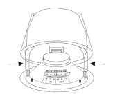
Pull down the speaker grill from the red fire dome. Disconnect the grill from the fire dome by compressing the 2 spring connections
