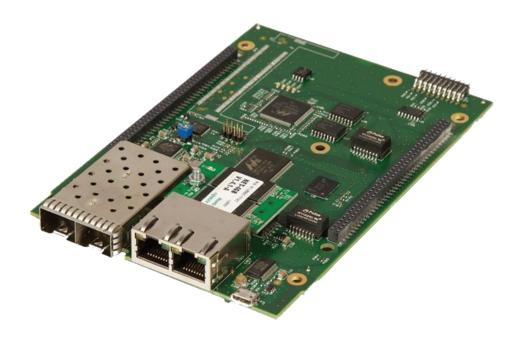
The optional EF-VIPEDIA-NET card plugs on to the main EFDAU2000 board, adding network interface ports and IP network audio channels to the base EFDAU2000 unit and increasing the maximum system size. EF-VIPEDIA-NET is usually installed to provide large multi-channel distributed Voice Alarm Systems.
