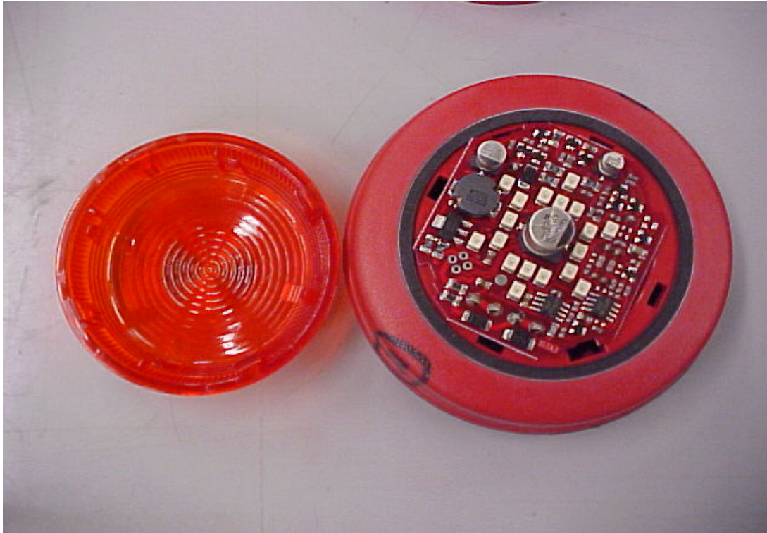
No ingress of dust found inside Sample 2.
