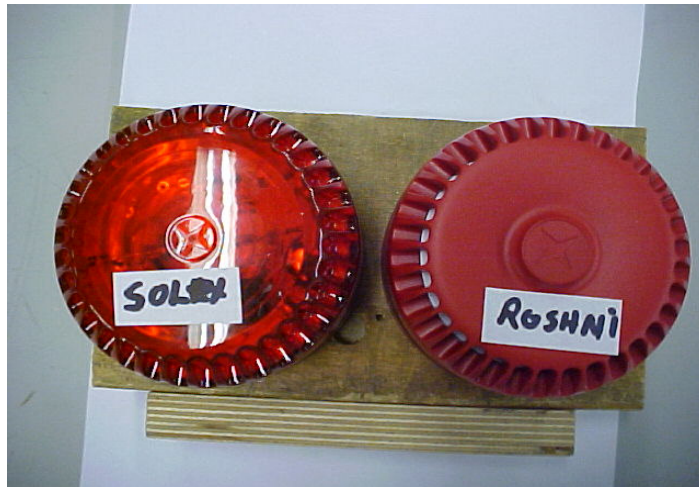
Samples during IPx4 water test
