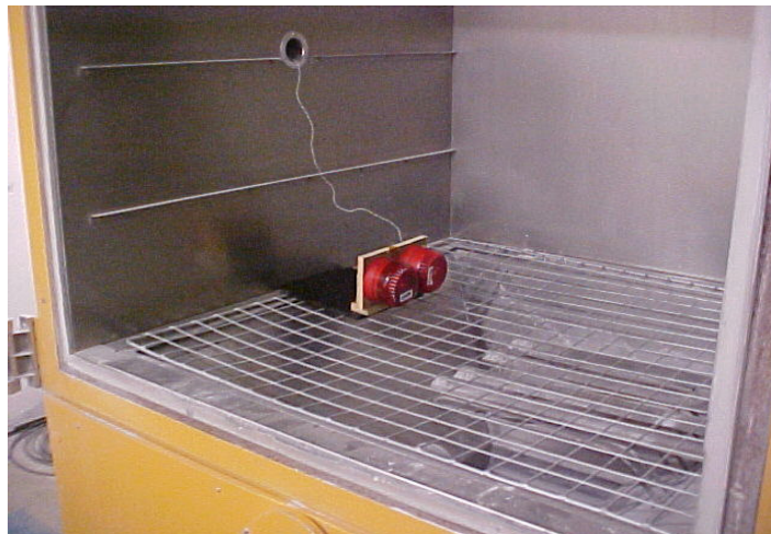
Samples at start of dust test
