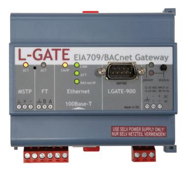
The BACnet gateway (EC650B) is a CEA-709/ BACnet gateway which maps CEA-709 network variables (NVs) to standard BACnet server objects. When ordered with this part code EC650B, the LonWorks to BACnet address mapping is preloaded and ready for use with the Eaton intelligent addressable CF3000 system interface board.
