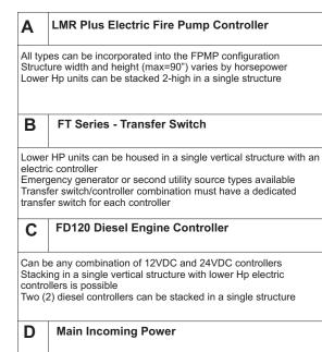
Can be connected directly to individual controllers which eliminates the need for a main switch / lugs - ideal for pump houses Non-Fusible Disconnect Switch, lockable in the ON position, can be supplied to power entire line-up
