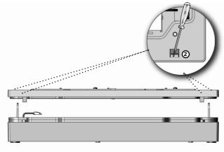
Press the legend-cover at the snap hooks together and remove it 0.
