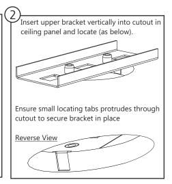
Screw in lower bracket but do not tighten until both lower and upper parts are parallel with the side of the ceiling tile. once parallel tighten screws. Ensure screws are not over tightened and damage ceiling tile.
