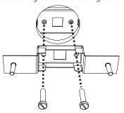
lower bracket. Secure in place with M5 nuts. Re-assemble fitting and refer to instruction K940 (supplied with fitting)
