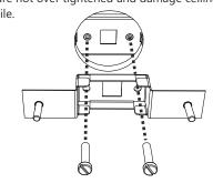
Locate Micropoint rear panel onto studs on lower bracket. Secure in place with M5 nuts. Re-assemble fitting and refer to instruction K940 (supplied with fitting)
